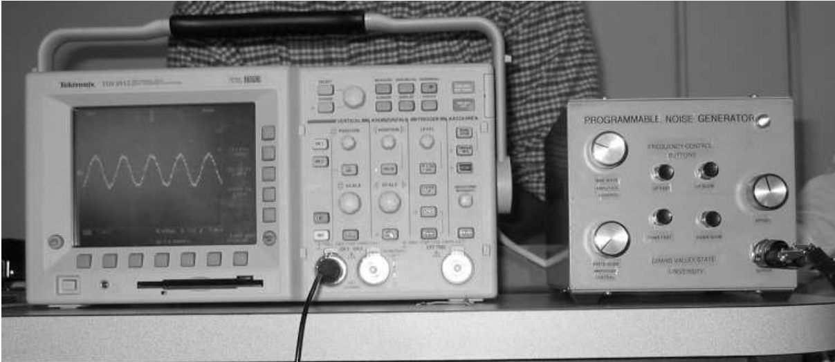
Figure 3: Photograph of the Sinusoidal Waveform Generator driving a sine wave into an oscilloscope
