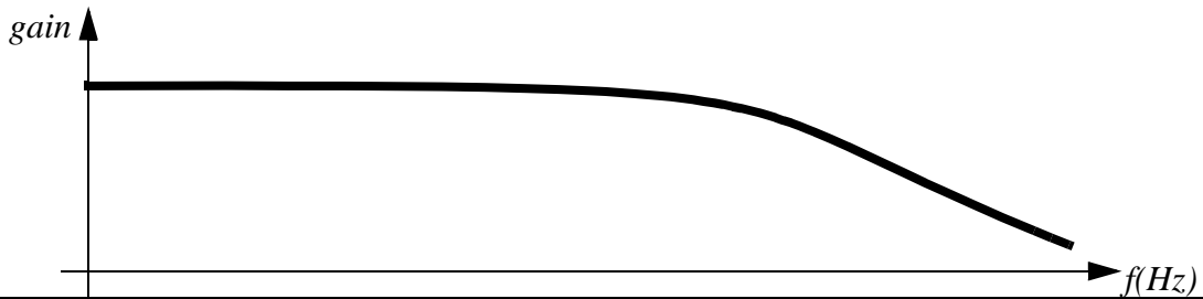
Figure 10.1 Commonly seen Bode plot
